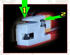
2-Slide the cable under the hook.
